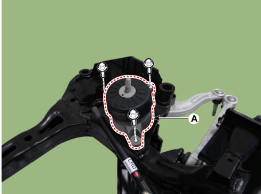
3. Remove the LH engine mounting support bracket (A).
