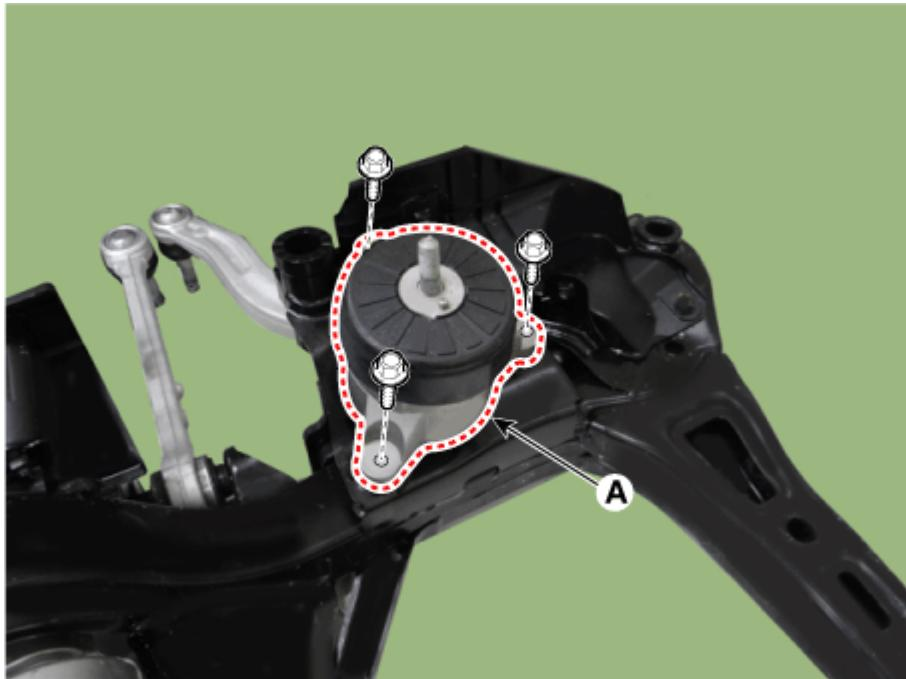
3. Remove the RH engine mounting support bracket (A).
