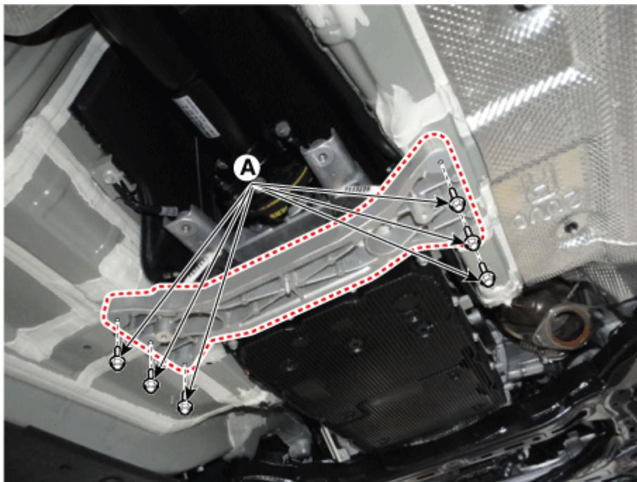
4. Remove the transmission mounting bracket (A).
